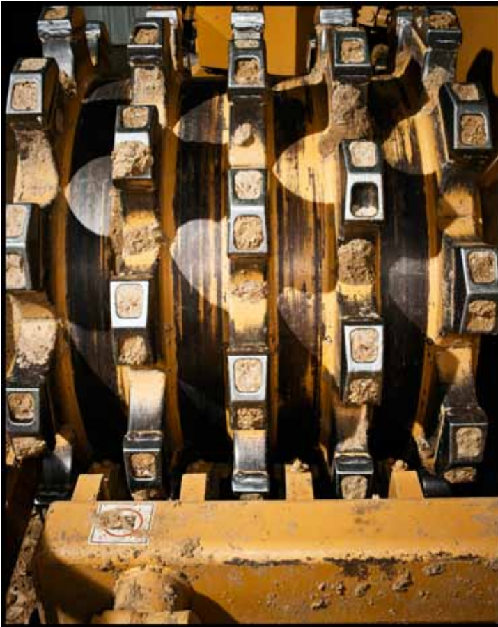
Below, a Caterpillar 992K wheel loader, which is 18 feet tall and weighs more than 200,000 pounds; left, the padfoot drum of a Cat soil compactor
